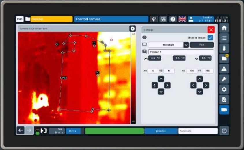
Integration of thermal imaging cameras for visual monitoring of injection moulded components and moulds
