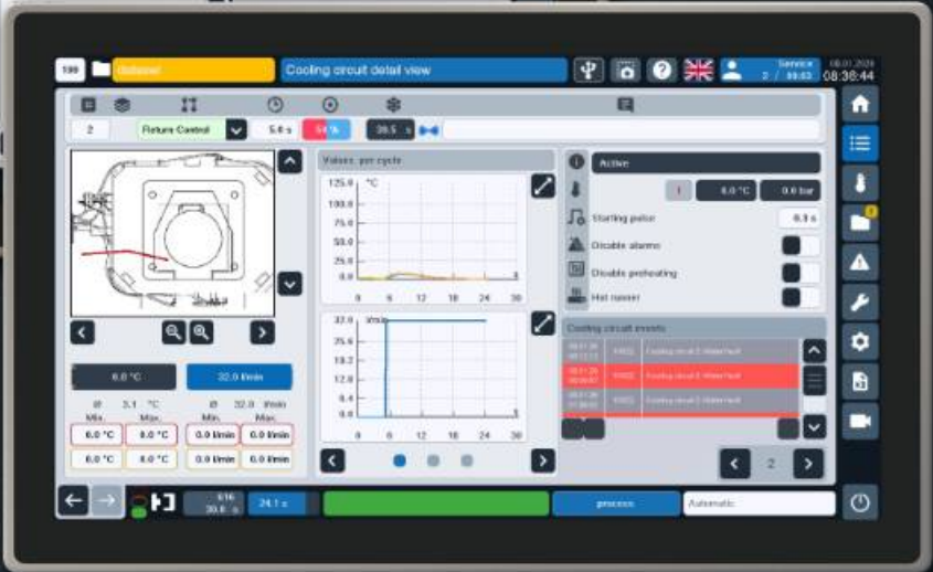
Integration of mould cooling plans Visualisation of all cooling circuits per mould side in a complete overview
